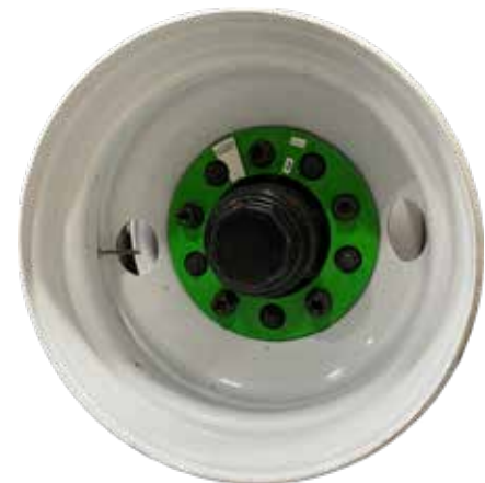
View of Loose Wheel Alarm installed
